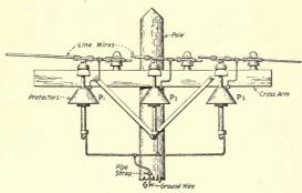
Fig. 167.—Outdoor-type, cupped-disc-gap protectors on a three-phase line.
